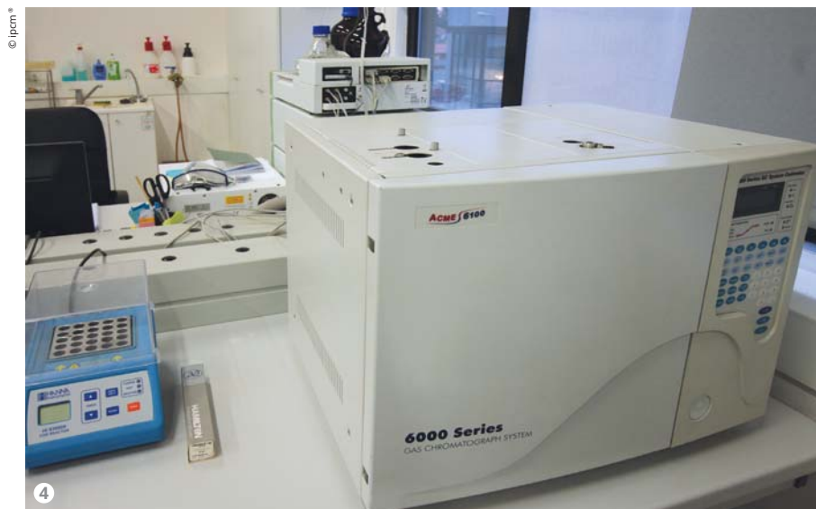
Figure 4: The gas chromatograph for the control of raw materials.
