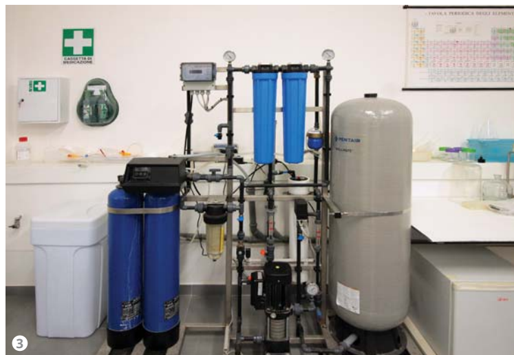
Figure 3: The Chemtec-branded 200 litre/hour reverse osmosis system with UV filters has been presented to the market recently.
