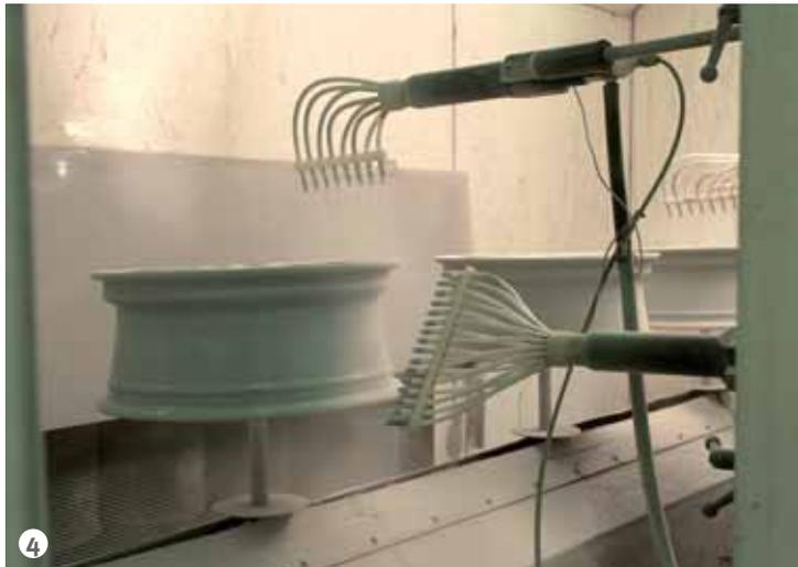
Figure 4: The application of the powder clearcoat.
