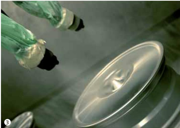
Figure 3: The application of the liquid coating with a robot.
