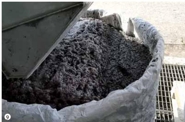
**Figure 9: The sludge container is replaced every two weeks and disposed of every six months.**
