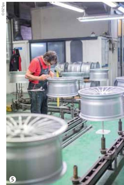
**Figure 5: The visual inspection after coating.**
